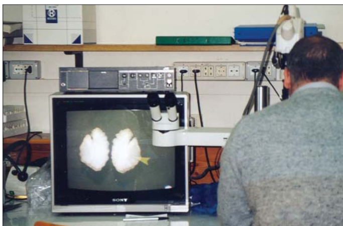
Fig. 1. Age determination of the red mullet, Mullus barbatus , in the nanism study, using otolith readings (seen on the monitor of the double station binocular)
